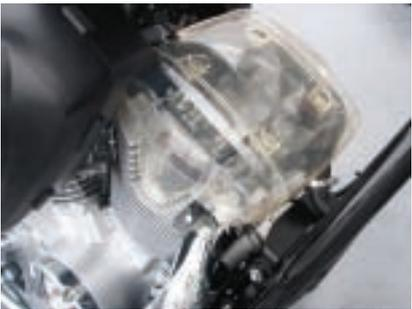
For the Fury and its patented radiator hose arrangement, this clear cylinder head cover was created to check final confirmation on clearances for the hose and also various internal parts.
