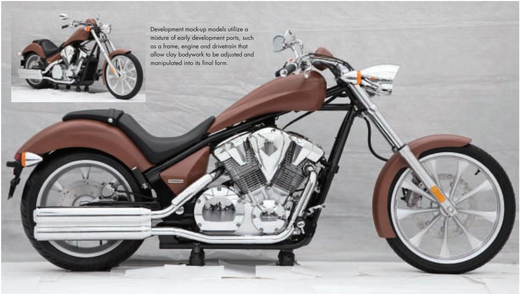
Development mock-up models utilize a mixture of early development parts, such as a frame, engine and drivetrain that allow clay bodywork to be adjusted and manipulated into its final form.
