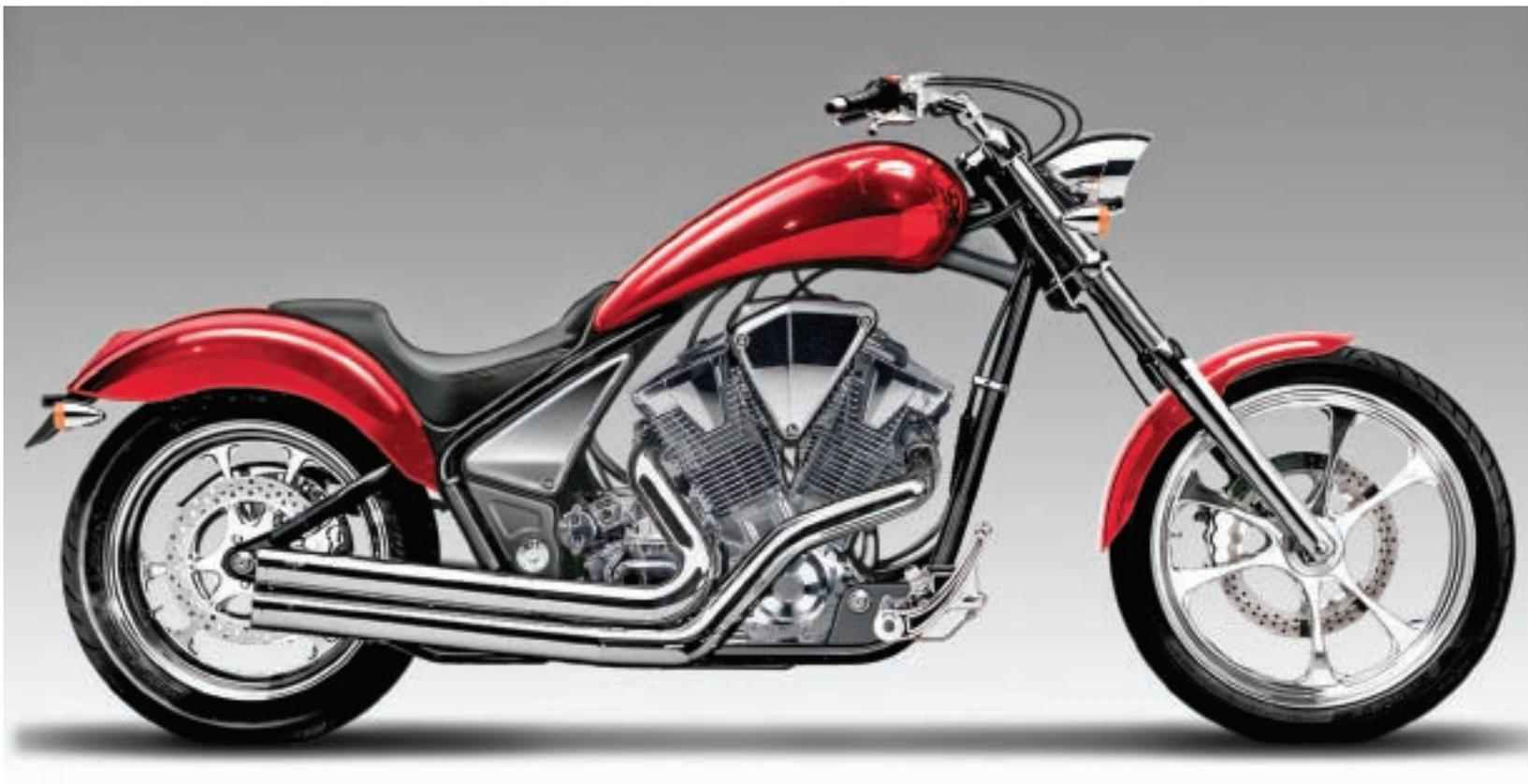
This is the first sketch of the Fury that kicked off the development process. As you can see, the overall proportion in this early sketch was preserved into production although the shapes were improved during the clay modeling process.
